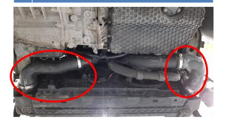
7. Disconnect the cable from its bracket on the intercooler inlet pipe. Then remove the pressure pipe from the car, remove it downwards.
