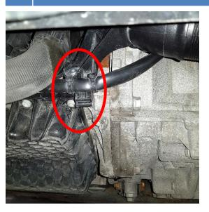
Remove the air intake scoop by removing 2x Torx T25 and unclick the radiator hose.
