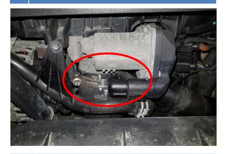
11. Install the OEM screws and rubber bushings (4pcs) from the OEM pipes on the do88 pipes. Also remove the sensor from the OEM pipe and install it in the do88 pipe with the included screws.
