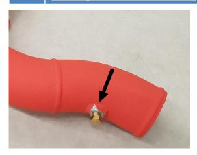
Put the turbo outlet hose on the other intercooler pipe, but don't tighten the clamp yet. Then install the pipe in the car. Just loosely tighten the two screws now.
