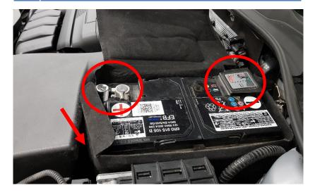
3. Loosen 1x Torx T30 screw at the pressure pipe bracket and 1x hose clamp on the turbo outlet. Also disconnect the small plastic box from it bracket on the battery tray.
