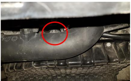
The do88 pipe comes with a 1/8 NPT meth injection connection. If you don't want to use this install the included blanking bung. Screw it in carefully with some lubrication!
