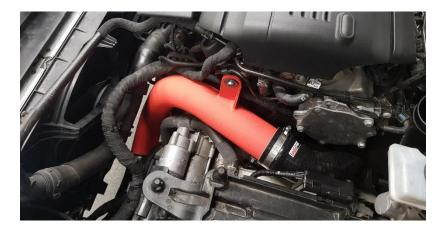
Put the throttle body hose on the intercooler pipe, but don't tighten the clamp yet. Then install the pipe in the car. Just loosely tighten the two screws now.
