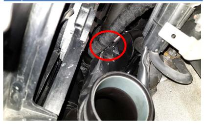
6. Disconnect the cable from its bracket on the intercooler inlet pipe also loosen 1x Torx T30.
