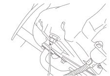
Screw the oil drain plug back to the oil return pipe.
